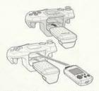
When the Vibration Pack is inserted into Expansion Socket 1 of the Sega Dreamcest Controller, the Vibration Pack does not lock into place and may fall out during game play or otherwise inhibit game operation. To return to the title screen of any point during game play, simultaneously press and hold the A, B, X, Y, and Start buttons. This will cause the Seau Dreamcest to soft-reset the software.
